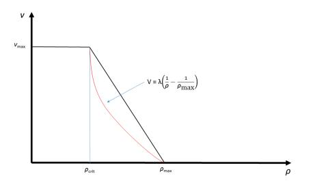
Figure 1: Original (in red, from [7]) and simplified flux curves illustrating speed-density relationship.
