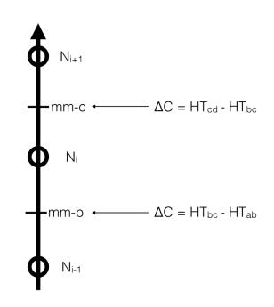
Figure 2: Schematic of *i*th road segment as a circular node. Here mm-x refers to mile-marker x, and  $\Delta C$  keeps track of the cars that have entered or exited the road between nodes.
