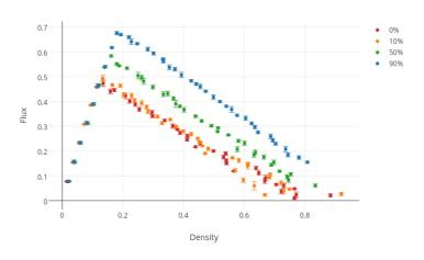
Figure 3: density and traffic flux data from our cellular automata model.
